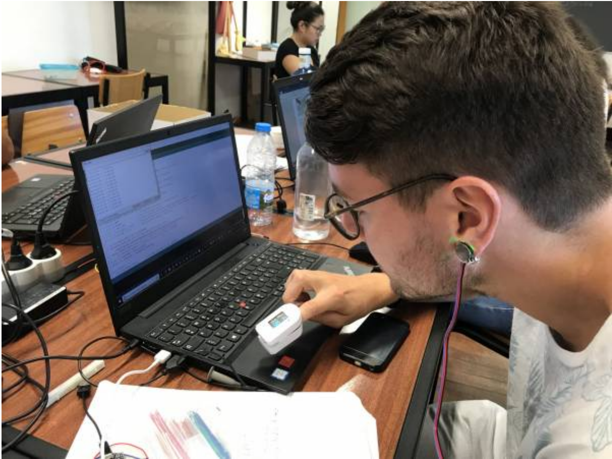
Figure 84: Pulse measurement with earclip and reference Fingermeasurement
