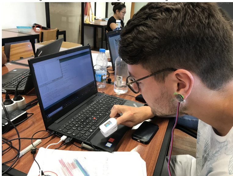
Figure 82: Pulse measurement with earclip and reference Fingermeasurement
